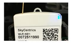
2. Insert Paper clip into the hole at top edge of DC module, and push gently on Factory Reset button for over 7 seconds until LED goes OFF.
