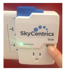
3. The plug will reboot and power up and be factory reset and ready in about 10-20 seconds, at which time it will broadcast its "CB xxxxxx" Wi-Fi address and you can connect it to the Wi-Fi network of your choice.
