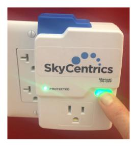
2. Hold the button down for over 7 seconds until LED goes OFF, and then release.
